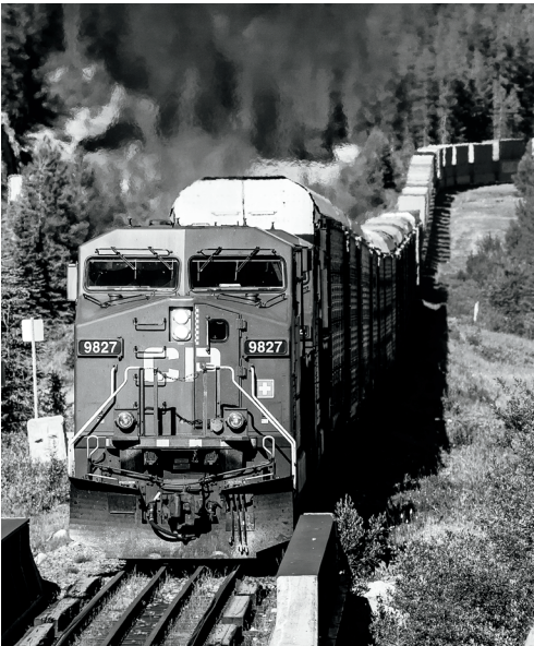
AC 4400CW locomotive 9827, heads a westbound freight about to cross the Blue Creek bridge east of Wapta Lake. The locomotive has just pulled through the "Hector Dip" – so named for the old siding that was nearby. This uphill on a downhill (vice-versa for eastbound trains) requires that a locomotive engineer pay close attention to the power requirements and train speed. As you can see, the head end of the train is climbing while, 20 cars back, the consist is descending.
