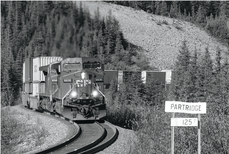
Two AC4400CW locomotives, 9836 assisted by 8549, power an eastbound intermodal "stack" train up the Field Hill, 1 mile east of Partridge siding, June 1, 2008. The sign indicates mile 125.7 of the Laggan Subdivision, as measured from Calgary. 9836 was delivered to CP in 2004. 8549 was in the first batch of AC4400CWs, delivered in 1998. These units, and the one pictured below, will be among the last of their model to be converted to AC4400CW(M), or otherwise rebuilt or retired.
